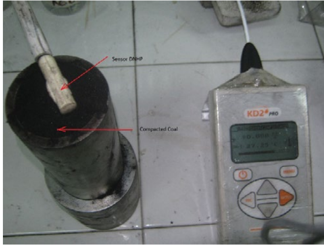
Figure 2. Measurement of the thermal conductivity of carbon powder by means of the KD2 PRO® equipment. Ceramic Materials Research Center CIMAC. Francisco de Paula Santander University.
