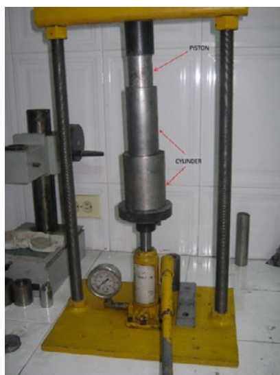
Figure 1. Thermal carbon powder compaction pressure system. Ceramic Materials Research Center CIMAC. Francisco de Paula Santander University.
